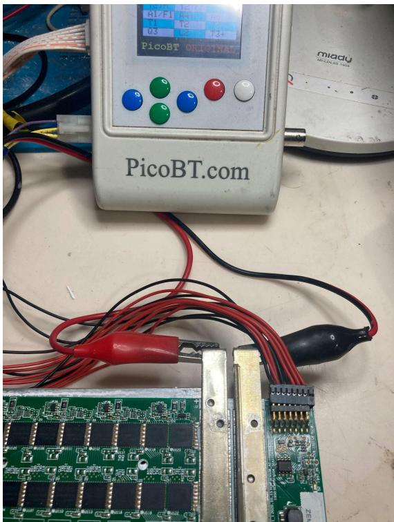
5. Run the diagnosis tool, it should read the number of chips and the board batch number.
