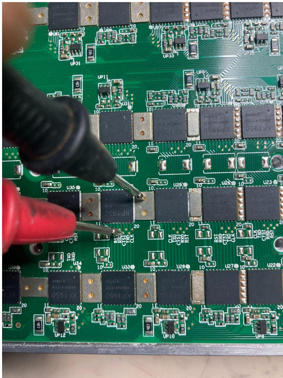
13. If the boost and the LDOs are okay, measure the individual signals on the chipset. They should match up as below.
