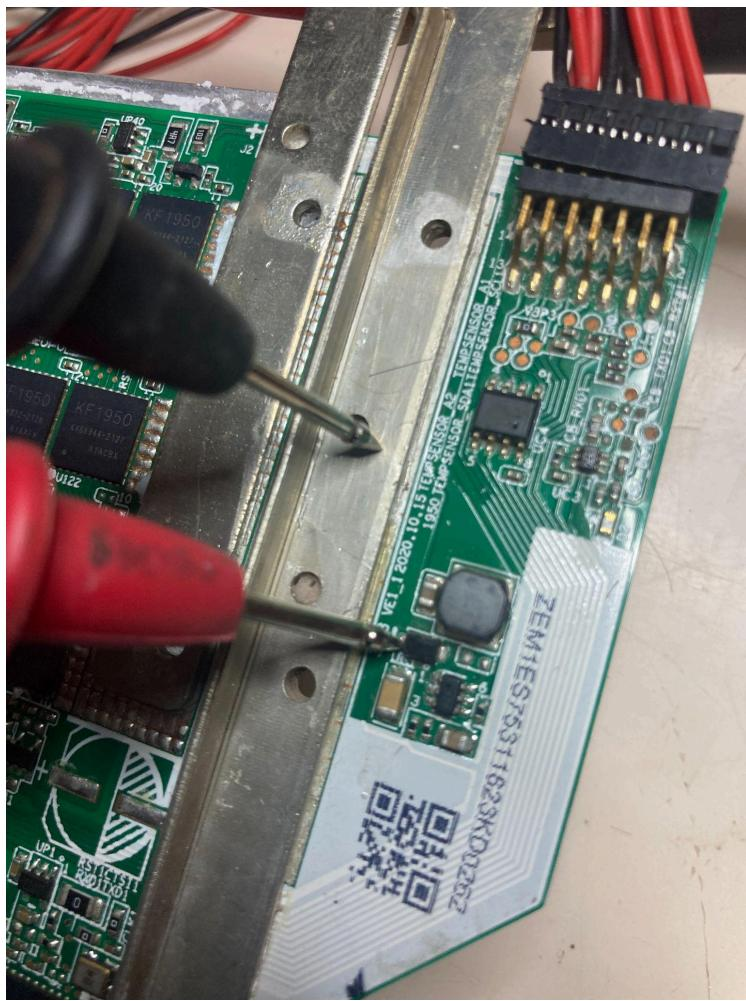
8. If the boost output voltage is below the value indicated above, replace the boost as per the Boost replacement instructions below.
