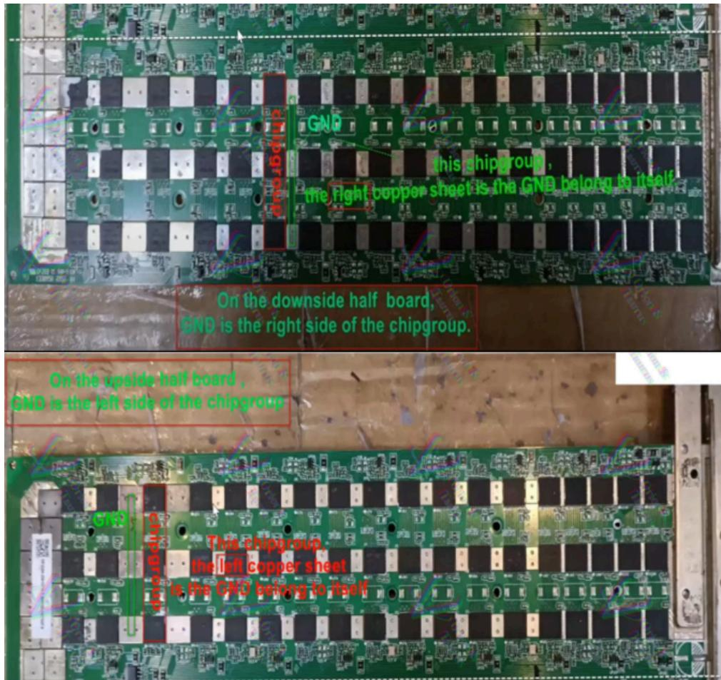
12. If any of the LDO output voltage is below the value indicated above, replace the LDO as per the LDO replacement instructions below.
